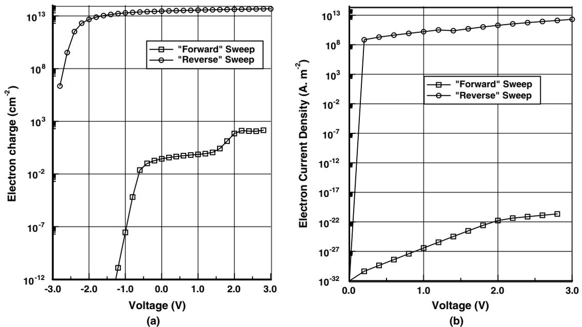
Fig. 1. (a) Charge control results for the diode structure. The charge shown is the electron charge in the GaN channel region of the device. In the “reverse” sweep, the charge induced is orders of magnitude higher than it is under the “forward” sweep. (b) Forward bias characteristics for the diode structure. The current almost completely shuts off in the “forward” sweep. In the “reverse” sweep, this current shows nearly classic diode behaviour.
