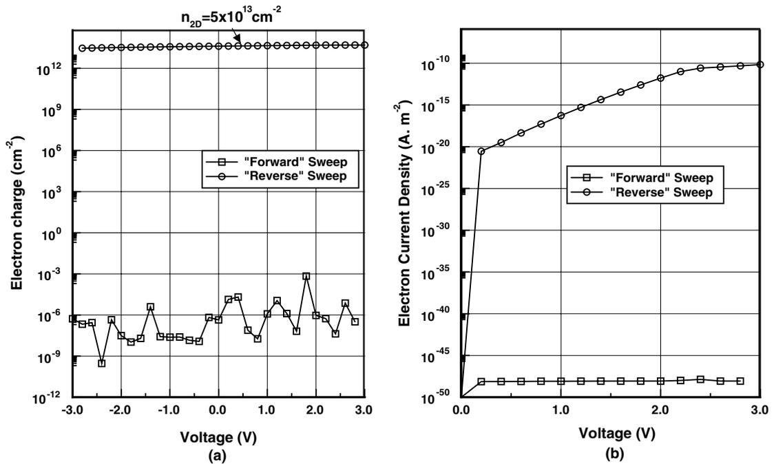
Fig. 2. (a) Charge control results for the undoped high sheet charge structure. The charge shown is the electron charge in the GaN region as before. The difference in the charge induced in the two sweeps is even greater than it is in Fig. 1. (b) Forward bias characteristics for the structure. In both sweeps, the vertical tunneling current is extremely low.
