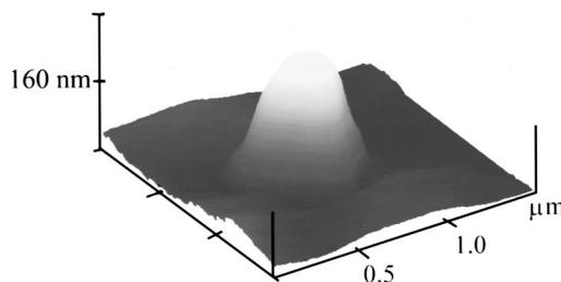
FIG. 4. AFM image of a submicron diamond indenter fabricated by FIB lithography.
