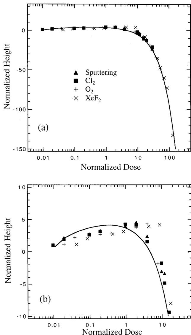
FIG. 3. (a) Normalized height vs normalized dose for various assisting gases and physical sputtering. Solid curve is the fitting of Eq. (3) to the results of physical sputtering and Cl<sub>2</sub>-assisted etching. (b) Details of (a) showing the deviation in the medium-dose range for gases O<sub>2</sub> and XeF<sub>2</sub> from the universal behavior.
