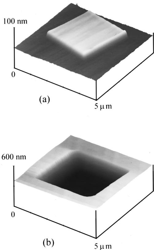
FIG. 1. AFM image of (a) a mount created by FIB bombardment (dose  $1 \times 10^{17}$  ions/cm<sup>2</sup>) and (b) a crater created by XeF<sub>2</sub>-assisted FIB etching (dose  $1 \times 10^{18}$  ions/cm<sup>2</sup>).
