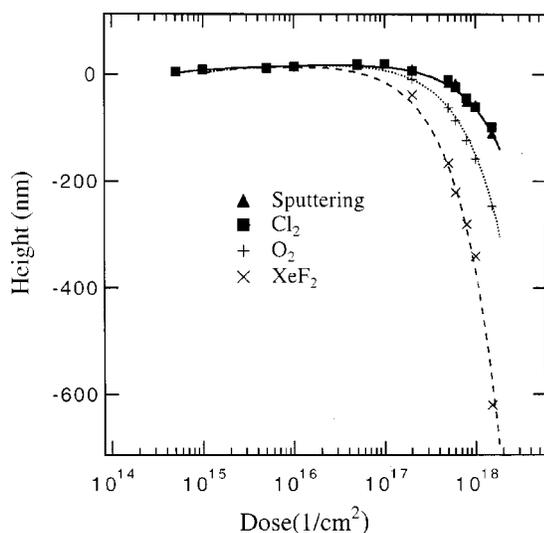
FIG. 2. Height of the bombarded area vs ion dose for various assisting gases and physical sputtering.
