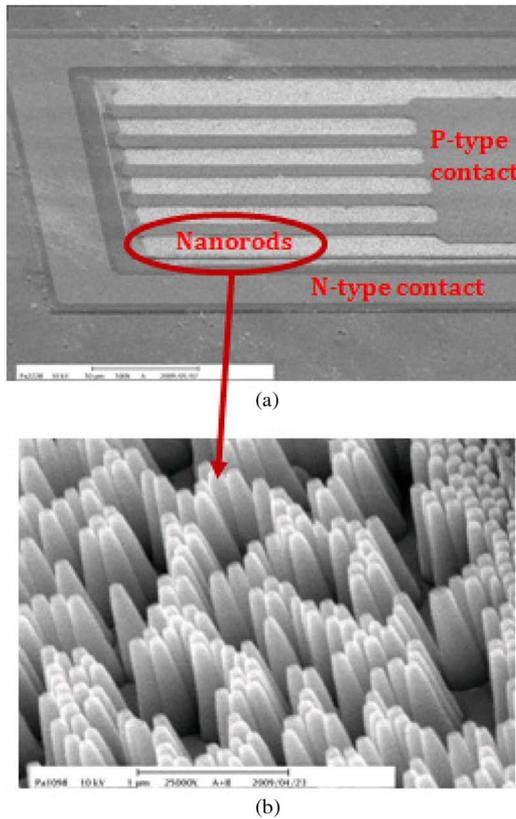
Fig. 2. (a) Top view image of the LED with nanorods and (b) close-up view of the nanorods.
