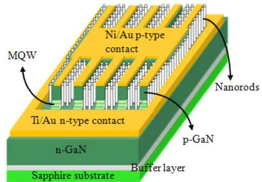
Fig. 1. Illustration of the device profile of an LED encompassed with nanorod arrays.
