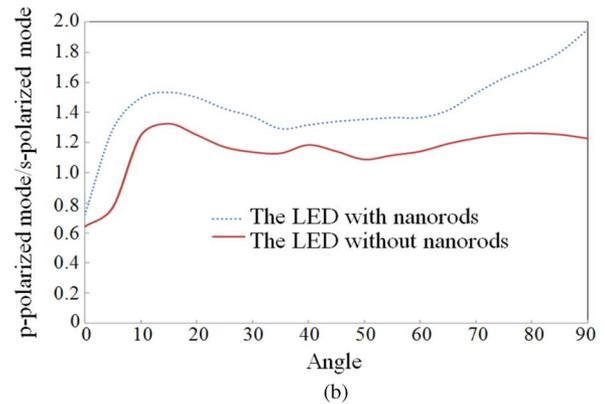
Fig. 4. (a) Radiation profiles of the devices with and without nanorods biased at an injection current 1 mA. (b) The p/s-polarized ratios at various radiated angles.
