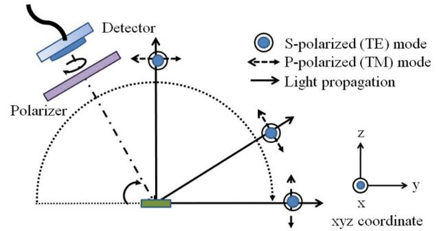
Fig. 3. Experimental setup for angular dependent polarized light measurement. Directions of p- and s-polarized light and the  $xyz$  coordinate are also indicated.
