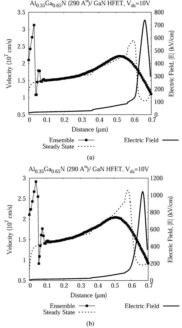
Fig. 3.  $L_g = 0.70\ \mu\text{m}$ . Ensemble Monte Carlo channel velocity profile, the corresponding steady-state velocity profile calculated from the velocity field relations [6], and the electric field in the channel for (a)  $V_{\text{gs}} = -2\text{ V}$  and (b)  $V_{\text{gs}} = -4\text{ V}$ .
