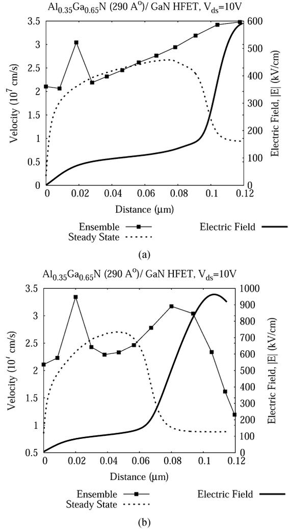
Fig. 5. Electric field and channel velocity profile results for  $L_g = 0.12\ \mu\text{m}$  for (a)  $V_{gs} = -2\ \text{V}$  and (b)  $V_{gs} = -4\ \text{V}$ .
