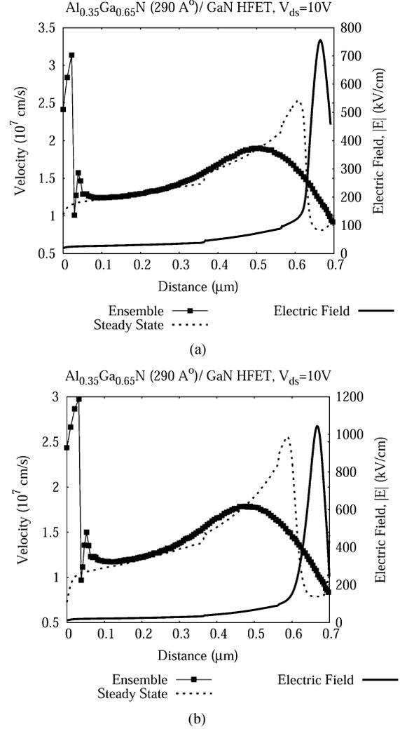
Fig. 10. Electric field and channel velocity profile results for  $L_g = 0.70 \mu\text{m}$  at 400 K for (a)  $V_{gs} = -2 \text{ V}$  and (b)  $V_{gs} = -4 \text{ V}$ .
