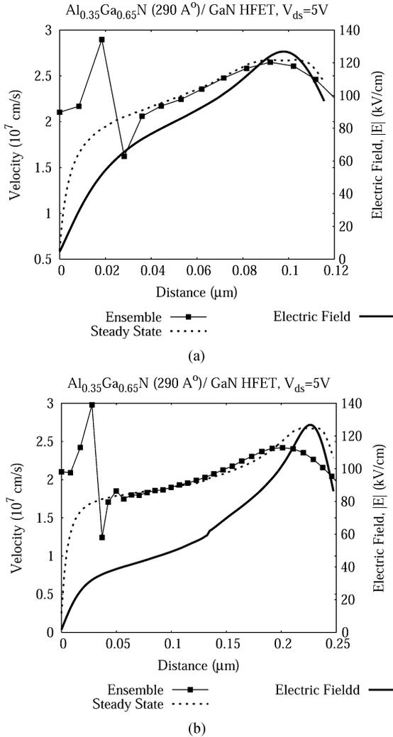
Fig. 6. Electric field and channel velocity profile results for  $V_{gs} = -2$  V,  $V_{ds} = 5$  V for (a)  $L_g = 0.12$   $\mu\text{m}$  and (b)  $L_g = 0.25$   $\mu\text{m}$ . Velocity overshoot appears to be suppressed for these bias conditions.
