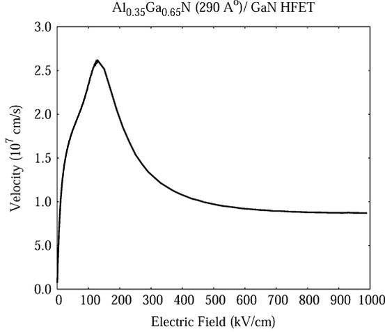
Fig. 2. Steady-state velocity-field characteristics for the  $\text{Al}_{0.35}\text{Ga}_{0.65}\text{N}$  structure shown in Fig. 1 at  $T = 300\text{ K}$  and for a gate bias of 0 V.
