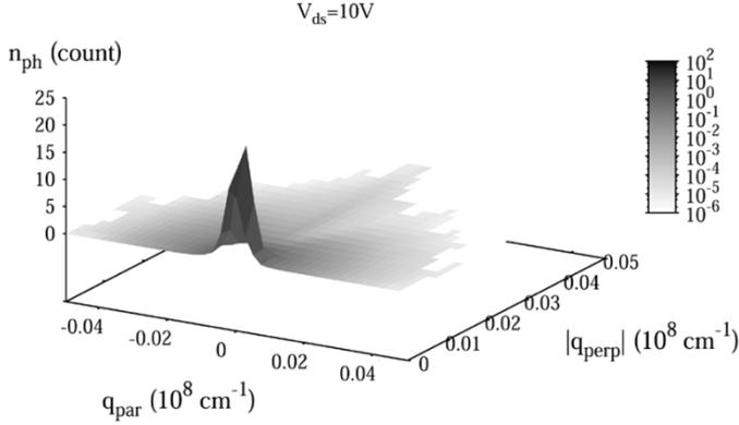
Fig. 8.  $L_g = 0.12 \mu\text{m}$ . Momentum spectrum of ensemble averaged polar optical phonon count per electron for  $V_{gs} = -2 \text{ V}$ . As in Fig. 7, the Monte Carlo simulations are carried out over a region much larger than the gate area.
