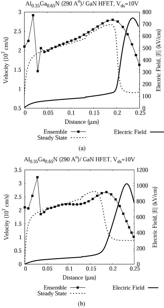
Fig. 4. Electric field and channel velocity profile results for  $L_g = 0.25\ \mu\text{m}$  for (a)  $V_{gs} = -2\ \text{V}$  and (b)  $V_{gs} = -4\ \text{V}$ .
