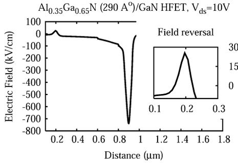
Fig. 9.  $L_g = 0.70 \mu\text{m}$ . Electric field profile obtained through a finite element method for  $V_{gs} = -2 \text{ V}$ . The inset shows the region of field reversal in greater detail.
