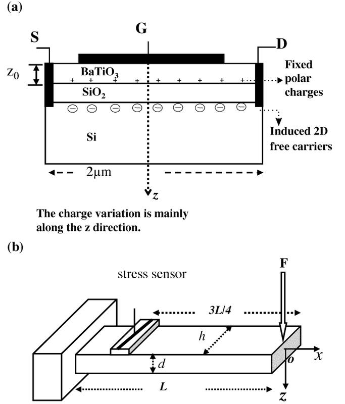
Fig. 4. (a) Schematic of the MPISFETs structure. The gate length is  $1 \mu\text{m}$ . (b) MPISFETs is assumed to be grown on top of the cantilever.  $L$  is the total length of the cantilever which is set to be  $200 \mu\text{m}$ .  $d$  is the height of the cantilever, which is set to be  $10 \mu\text{m}$ .  $O$  is the origin of the Cartesian coordinate. The sensor FET is at  $x = 3/4L$ .
