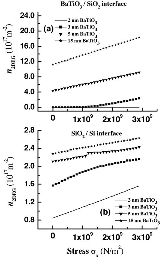
Fig. 5. Calculated sheet charge density, ( $n_{2DEG}$ ), at the Si-SiO<sub>2</sub>-BaTiO<sub>3</sub> heterostructure junctions. (a) The  $n_{2DEG}$  at the SiO<sub>2</sub>-BaTiO<sub>3</sub> interface; and (b) the  $n_{2DEG}$  at the Si-SiO<sub>2</sub> interfaces. The SiO<sub>2</sub> layer thickness is 8 Å. The gate voltage is 0 and the Schottky-barrier height is taken to be 1.5 eV.
