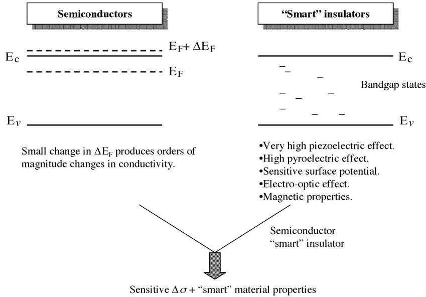
Fig. 1. Semiconductors have the remarkable properties of conductivity and  $e - h$  injection control. Smart materials based on various oxides have remarkable polarization, magnetic, and electrooptic properties. The heterostructures between the two classes would lead to novel devices.
