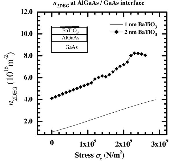
Fig. 8. Calculated sheet charge density, ( $n_{2\text{DEG}}$ ), at the GaAs–Al<sub>0.3</sub>Ga<sub>0.7</sub>As heterostructure interface. The thickness of Al<sub>0.3</sub>Ga<sub>0.7</sub>As layer is 40 Å. The gate voltage is 0 and Schottky-barrier height is taken to be 1.5 eV.
