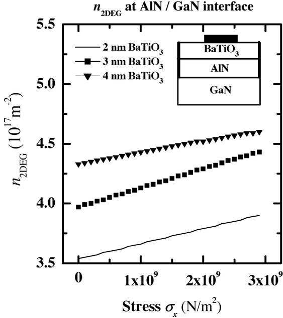
Fig. 7. Calculated sheet charge density, ( $n_{2\text{DEG}}$ ), at the GaN–AlN heterostructure interface. The thickness of AlN layer is 30 Å. The gate voltage is 0 and Schottky-barrier height is taken to be 1.2 eV, respectively.
