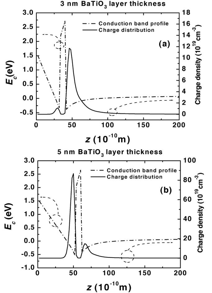
Fig. 6. Calculated charge density and conduction band profiles of Si-SiO<sub>2</sub>-BaTiO<sub>3</sub> heterostructure junctions. (a) 30 Å BaTiO<sub>3</sub> layer thickness under stress  $\sigma_x = 10^9 \text{ N/m}^2$ , and (b) 50 Å BaTiO<sub>3</sub> layer thickness under the same stress  $\sigma_x = 10^9 \text{ N/m}^2$ . The SiO<sub>2</sub> layer thickness of is 8 Å. The gate voltage is 0 and Schottky-barrier height is taken to be 1.5 eV.
