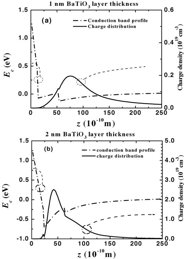
Fig. 9. Calculated charge density and conduction band energy profiles of GaAs–AlGaAs–BaTiO<sub>3</sub> heterostructure junctions. (a) 10 Å BaTiO<sub>3</sub> layer thickness under stress  $\sigma_x = 10^9 \text{ N/m}^2$ ; and (b) 20 Å BaTiO<sub>3</sub> layer thickness under stress  $\sigma_x = 10^9 \text{ N/m}^2$ . The gate voltage is 0 and Schottky-barrier height is taken to be 1.2 eV.
