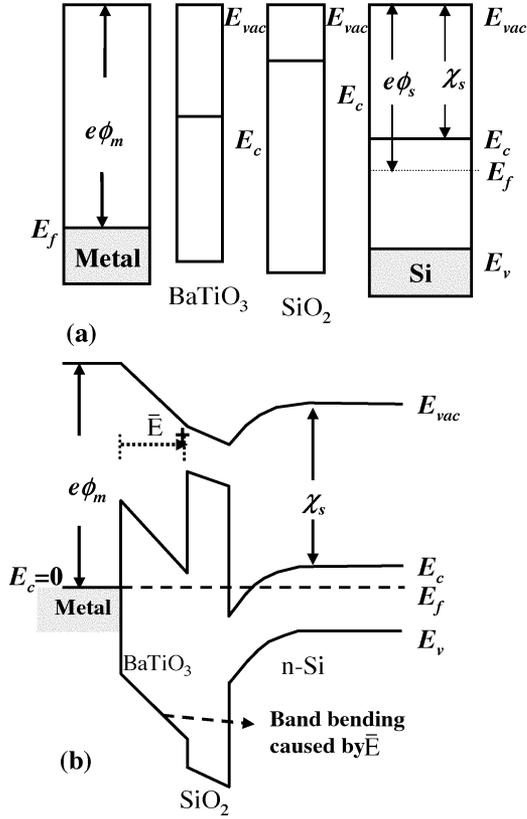
Fig. 3. (a) Band profiles of the isolated metal, the polar oxide, the oxide, and the semiconductor.  $\phi_m$  is metal work function,  $\chi_s$  is the electron affinity,  $E_{vac}$  is the vacuum energy level,  $E_c$  is the conduction energy band,  $E_v$  is valence band, and  $E_f$  is the Fermi-level. (b) Band profile of the heterostructure junctions.
