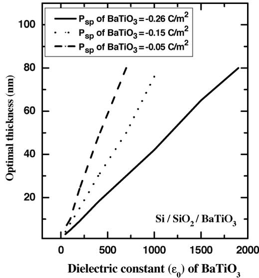
Fig. 11. Calculated optimal BaTiO<sub>3</sub> layer thickness of Si-SiO<sub>2</sub>-BaTiO<sub>3</sub> heterostructure sensor-FETs for different dielectric constants and spontaneous polarization. The thickness of SiO<sub>2</sub> layer is 8 Å. The gate voltage is 0 and Schottky-barrier height is taken to be 1.5 eV. As discussed in the text, at the optimal thickness the 2DEG is located at the SiO<sub>2</sub>-Si interface.
