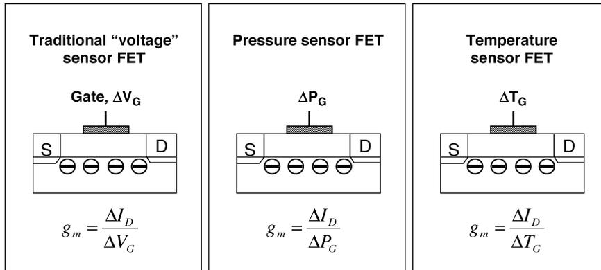
Fig. 2. Schematic of smart sensors based on oxide–semiconductor heterostructures.
