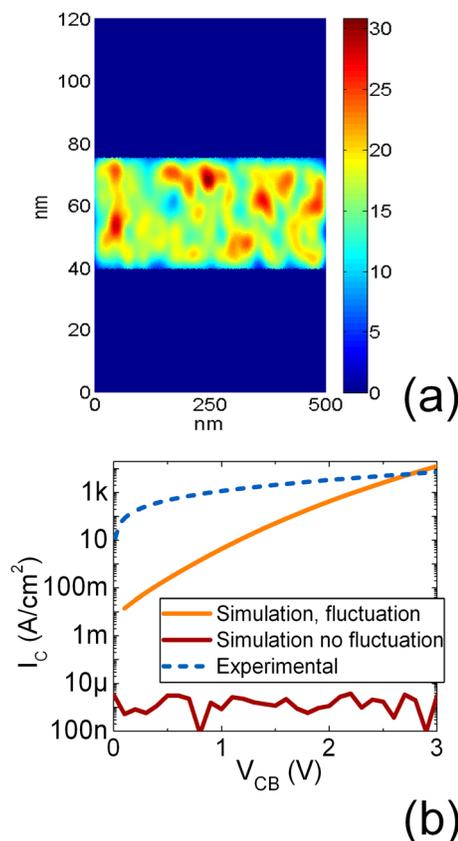
FIG. 2. (a) Modeling of statistical fluctuations of Al-composition in ternary  $\text{Al}_{0.20}\text{Ga}_{0.80}\text{N}$  layer. (b) Comparison of measured leakage current densities with those estimated from 2D FEM drift-diffusion transport with and without incorporating statistical fluctuations of Al-composition.
