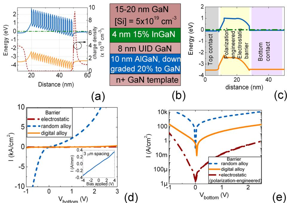
FIG. 3. (a) Energy band diagram of the sample D1 with a digital AlGaIn barrier. (b) Epitaxial stack of the sample with polarization-engineered binary GaN barrier. (c) Energy band diagram of the same. Comparison of measured leakage for samples with random alloy, binary GaN, and digital alloys as barriers in (d) linear (e) log scale. Inset to Figure 3(d) shows the lateral I-V between two top-contacts of the same device indicating its linear and Ohmic nature (the digital alloy sample).
