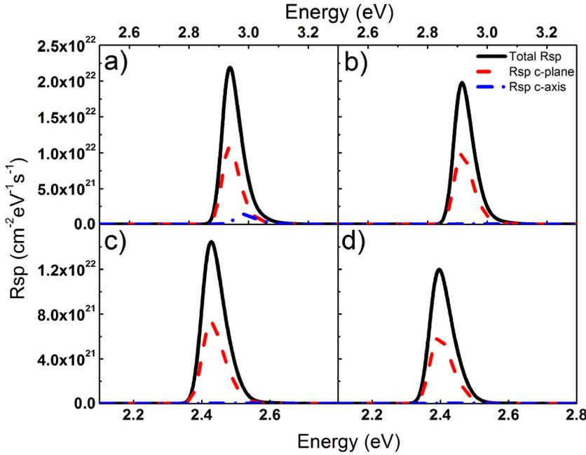
FIG. 4. Spontaneous emission spectra at injection carrier density equal to  $2.5 \times 10^{12} \text{ cm}^{-2}$  for both the blue ( $x = 14\%$ ) and green ( $x = 26\%$ ) LED structures having  $\text{In}_x\text{Ga}_{1-x}\text{N}/\text{GaN}$  quantum wells with metamorphic layer ((a) and (c)) and the conventional quantum well structure ((b) and (d)).
