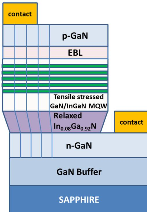
FIG. 3. Proposed *c* plane InGaN LED device structure using a metamorphic layer before the MQW region which is grown on the top of *n*-type GaN layer. The InGaN quantum well has either 14% or 26% for the blue or green emission, respectively.
