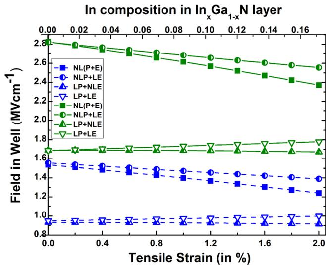
FIG. 2. Dependence of the piezoelectric field in the well region as a function of tensile strain in the *c* plane, for both the blue and the green LED structures. We compare the calculations using the LP model, the NLP model, and the NLP model with the addition of NLE.
