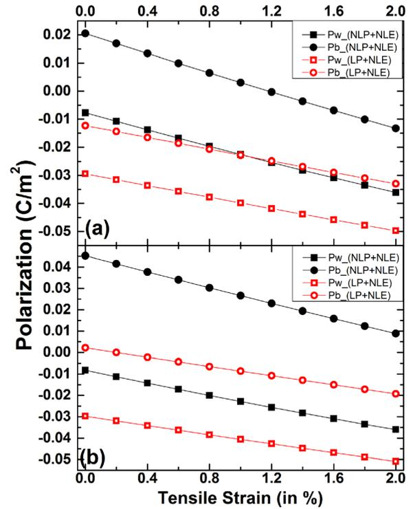
FIG. 1. Dependence of the total polarization (spontaneous plus strain induced polarization) in the well and barrier region as a function of tensile strain (evaluated from NLE) in the c-plane for both the blue (a) and the green (b) LED structures.
