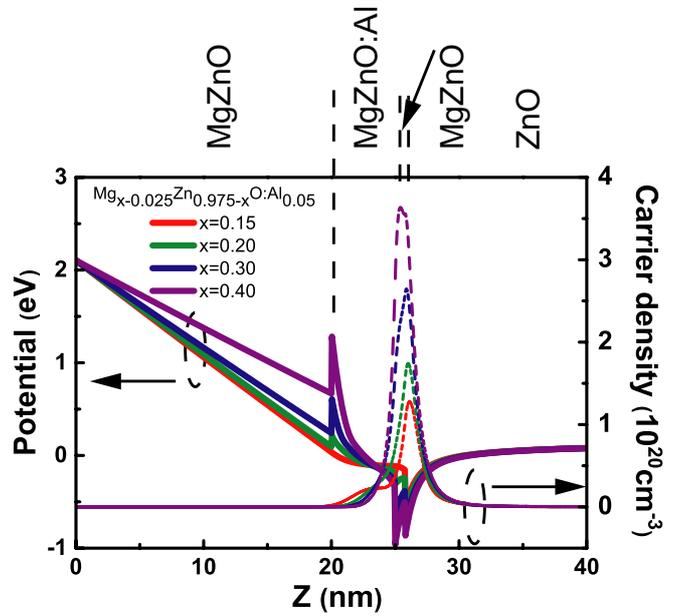
Figure 5. Simulation results for carrier and potential distributions in the heterostructure with a modulation doping layer of different Mg content. The composition of the barrier and capping layers is  $Mg_{0.15}Zn_{0.85}O$  and the composition of the modulation doping layer is  $Mg_{x-0.025}Zn_{0.975-x}O:Al_{0.05}$  with  $x = 15\%$ ,  $20\%$ ,  $30\%$  and  $40\%$ .
