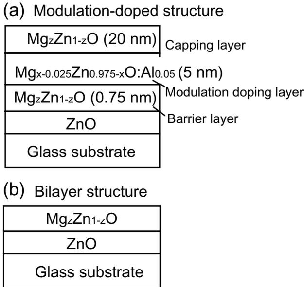
**Figure 1.** Schematics of (a) the modulation-doped structure and (b) the bilayer structure. The thickness of the  $Mg_zZn_{1-z}O$  layer in the bilayer structure is the saturation thickness indicated in [15].
