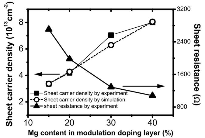
**Figure 2.** Sheet carrier density and sheet resistance of the heterostructure with modulation doping layer of different Mg content. The barrier and capping layers are  $Mg_{0.15}Zn_{0.85}O$  and the modulation doping layer is  $Mg_{x-0.025}Zn_{0.975-x}O:Al_{0.05}$  with  $x = 15\%$ ,  $20\%$ ,  $30\%$  and  $40\%$ . The closed symbols represent the experimental results, while the open symbols are the simulation results. The lines are drawn as a guide to the eye.
