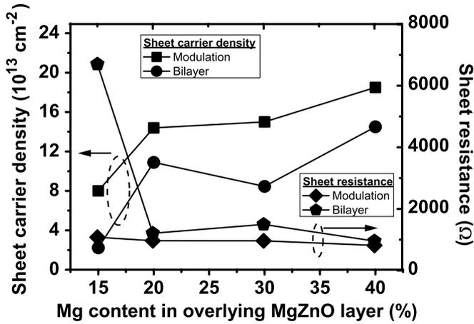
Figure 3. Sheet resistances and sheet carrier densities of the modulation-doped heterostructure and its counterpart, the bilayer heterostructure.
