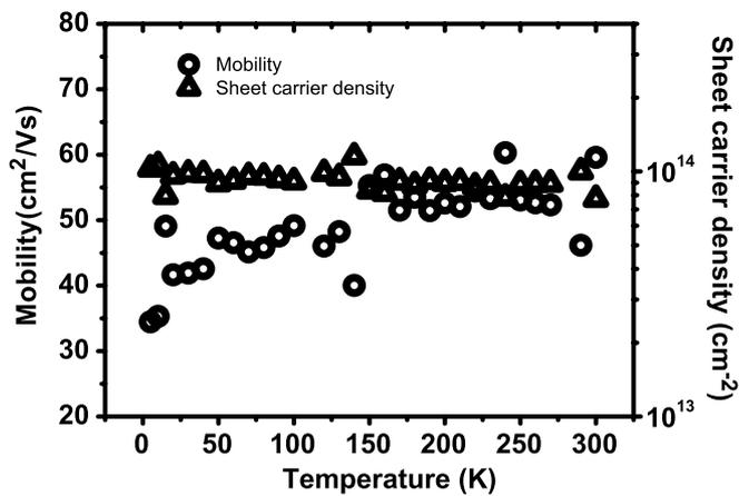
Figure 4. Hall mobility and sheet carrier density of the modulation-doped heterostructure as a function of temperature. The composition of the barrier and capping layers is  $Mg_{0.15}Zn_{0.85}O$ , and the composition of the modulation doping layer is  $Mg_{0.375}Zn_{0.575}O:Al_{0.05}$ .
