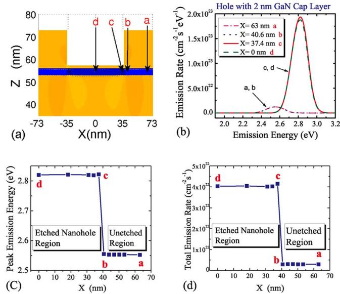
Fig. 4. (a) The strain distribution and the definition of a, b, c, and d points. (b) The calculated emission spectrum at a, b, c, and d points in 16 nm nanohole structure. Note that the curves for points a and b are almost overlapped and the curves for point c and d are also mostly overlapped. (c) The emission peak energy and (d) the total emission rate versus different positions for the 16 nm nanohole structure.
