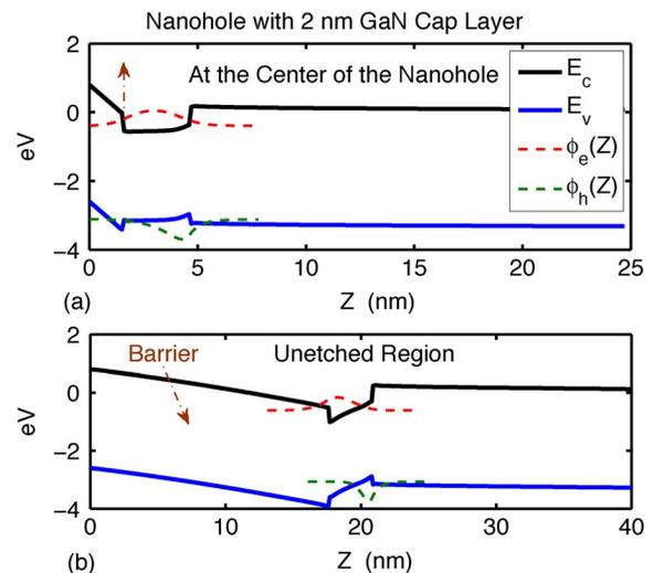
Fig. 3. The band structures and wavefunction of 16 nm nanohole structure at (a)  $X = 0.0$  nm (etched region) and (b)  $X = 64$  nm (unetched region).
