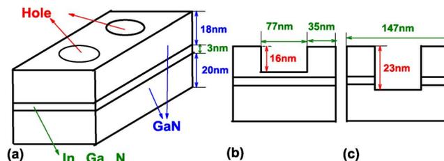
Fig. 1. A schematic of the nanohole structure. The hole depths are 16 nm and 23 nm.
