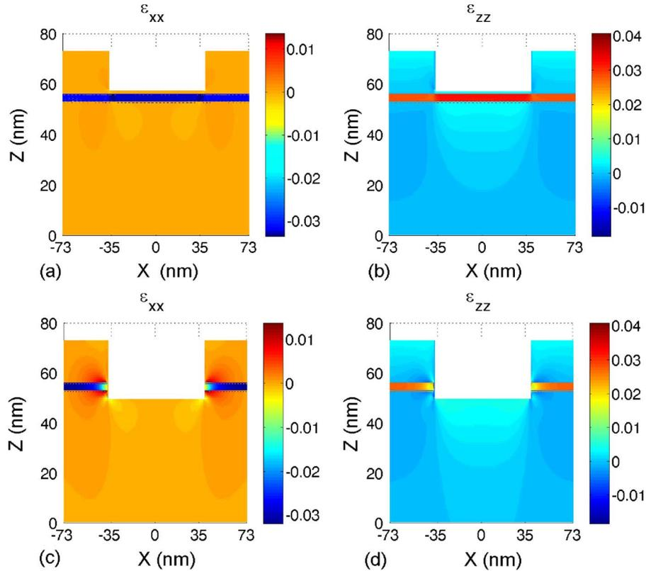
Fig. 2. The calculated strain tensor (a)  $\epsilon_{xx}$  and (b)  $\epsilon_{zz}$  of the nanohole structure with 16 nm hole depth. The calculated (c)  $\epsilon_{xx}$  and (d)  $\epsilon_{zz}$  of the nanohole structure with 23 nm-column hole depth.
