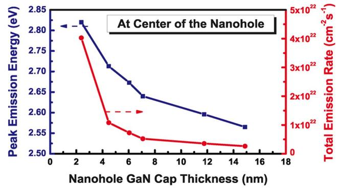
Fig. 5. The calculated emission strength and emission peak energy versus different nanohole GaN cap layer thickness (nanohole distance to the quantum well).
