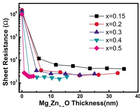
FIG. 2. (Color online) Sheet resistance of polycrystalline  $\text{Mg}_x\text{Zn}_{1-x}\text{O}/\text{ZnO}$  heterostructure vs thickness of  $\text{Mg}_x\text{Zn}_{1-x}\text{O}$  cap layer for  $x=0.15, 0.2, 0.3, 0.4,$  and  $0.5$ . The lines are guides to the eyes.
