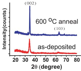
FIG. 1. (Color online) XRD pattern of rf-sputtered ZnO layer before and after 600 °C post-deposition annealing.
