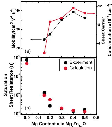
FIG. 3. (Color online) (a) Hall mobility and sheet carrier concentration of  $\text{Mg}_x\text{Zn}_{1-x}\text{O}/\text{ZnO}$  heterostructure in saturation as functions of Mg content  $x$ . (b) Comparison of experimental and calculated saturation sheet resistances as functions of Mg content  $x$ . The lines are guides to the eye.
