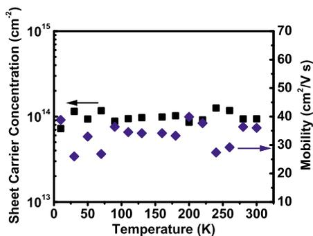
FIG. 4. (Color online) Hall mobility and carrier concentration of  $\text{Mg}_{0.3}\text{Zn}_{0.7}\text{O}/\text{ZnO}$  heterostructure with  $\text{Mg}_{0.3}\text{Zn}_{0.7}\text{O}$  capping layer thickness of  $\sim 30$  nm as functions of temperature.
