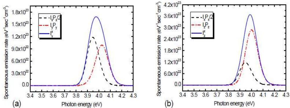
Fig. 4. (a) and (b) are the schematic illustrations of the influence of  $I_x P_x$  to the  $y$ -polarized light and  $z$ -polarized light, respectively.
