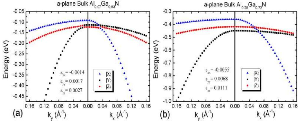
Fig. 3. The valence band energy dispersion relation under anisotropic tensile strained condition of the  $a$ -plane  $\text{Al}_x\text{Ga}_{1-x}\text{N}$  films (a)  $x = 0.07$  and (b)  $x = 0.28$ .
