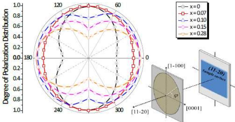
Fig. 2. The degree of polarization (DOP) of *a*-plane  $\text{Al}_x\text{Ga}_{1-x}\text{N}$  films with increasing Al composition  $x$  as a function of polarization angle starting at *c*-direction.
