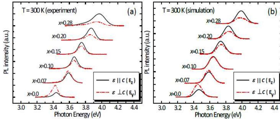
Fig. 1. (a) Experiment measurements and (b) simulation calculation of the PL intensity and spontaneous emission rate of *a*-plane  $\text{Al}_x\text{Ga}_{1-x}\text{N}$  films with the different aluminum compositions.
